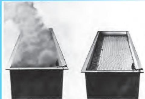
Floating cover balls are the simplest and most effective way to control:
